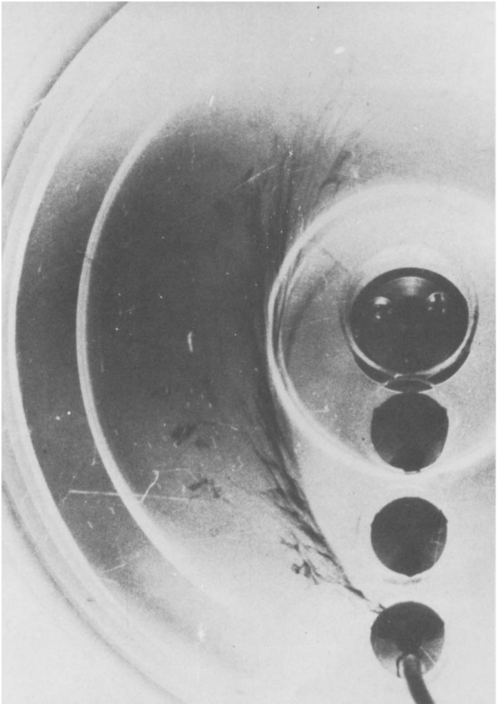
FIGURE 6. Photograph of dye streakline near plate surface in turbulent flow, \bar{R} = 16.9 .
